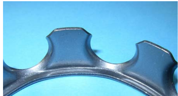
Figure 12. Superior formed cage design
